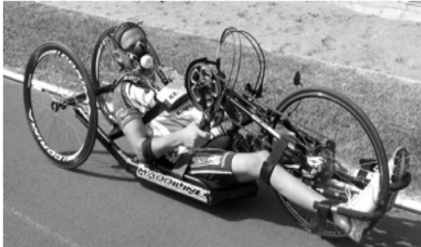
Figure 1. Handbiker equipped with a portable telemetric gas analysis system unit
